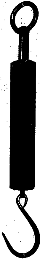
Fig. 38 Early Salter Spring Balance of 1770.
